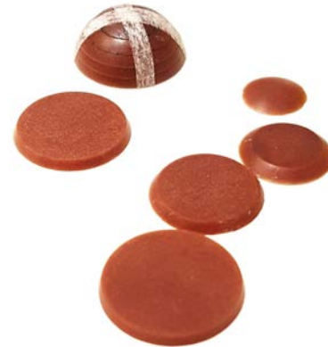
Figure 7 - Solid Water eyeball phantom for plaque measurements.
